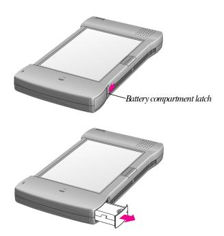
**3** Install four AA batteries in the battery compartment.
