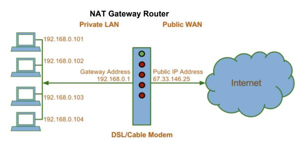
When a client on the private LAN requests an address located on the Internet, the request is forwarded to the NAT gateway. The gateway changes the source address of outgoing packets to match the IP address of the public facing (WAN Port) of the gateway. The router then forwards the outgoing packets further on to their destination over the Internet.
